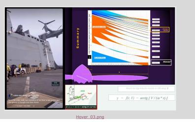
The propeller analyzed in the chart has a 2 m diameter, and has blades with a 30 degrees root-to tip twist. This is a little less than that of the proprotor blades of the V-22 with their 47,5 degrees. The 30 degrees ensures a 400 km/h design speed (axial) at a 2598 RPM. Rotational speed was chosen to produce a 0,8 Mach tip speed, in order to achieve some optimal propeller loss-ratio. (At 0,8 Mach classic equations of aerodynamics are considered to remain true yet.)
