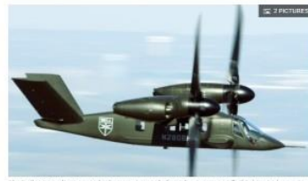
The Bell V-280 tiltrotor reached a true airspeed of 280 knots in a test flight this week. (Credit: Bell)
